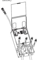
**6.** Place all wiring and connections back into the box and close the cover.
