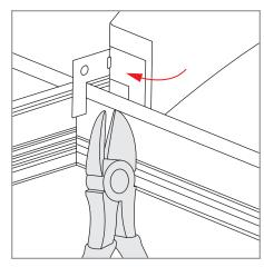
3. Use side cutters to adjust each tab to height of T-grid.
