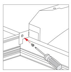
6. Use a #8 × 1/4" sheet metal screw (not supplied) to fasten fixture to T-grid.
