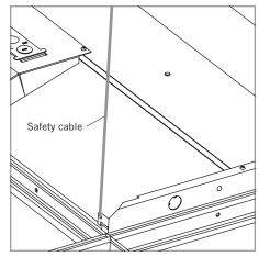
7. Use a safety cable (not supplied) to tie off in accordance with local building codes.
