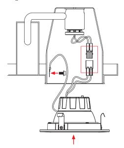
5. Carefully route wires into fixture, sliding the trim and friction clips into the housing for a tight fit.
