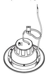
**4.** Plug E26 base cable connection into the recessed housing kit, ensuring that kit is grounded.
