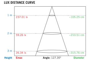
Note: The curves indicate the illuminated area and the average illumination when the luminaire is at a different distance.
