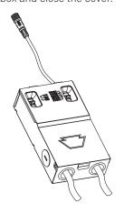
7. Insert driver box into ceiling in accordance with local/national codes and connect the male and female connectors. Screw threaded nut over connectors to secure.
