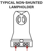
Connect wires directly to these terminals
