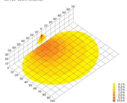
Ground mounted at 6" above ground, 10º above horizontal, shining towards building exterior
