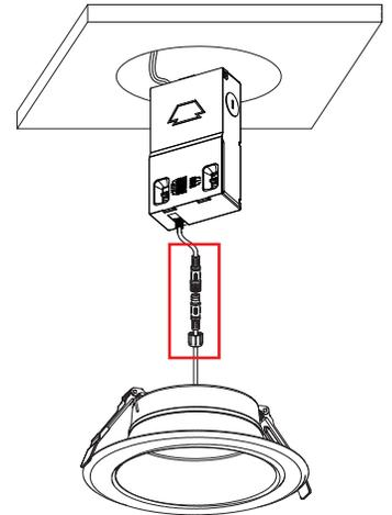
**8. Lifting both retention tabs upward, push the fixture into the hole until trim sits flush with ceiling.**
