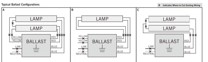
CAUTION: Use only non-shunted lampholders for Single-Ended wiring installations. Do not perform Single-Ended wiring installation of product in a fixture with shunted lampholders (found in all fixtures using instant start ballasts). If the existing lampholders are shunted, and Single-Ended wiring is desired, remove and replace them with non-shunted lampholders (or remove the external shunt if applicable). Make new connections directly to lampholder terminals as shown in Figure
