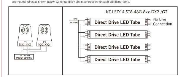
4. Complete all electrical connections with appropriate connectors/wire nuts as needed, per all local and national electrical codes. NOTE: There should not be any exposed wires from sockets left unconnected.
