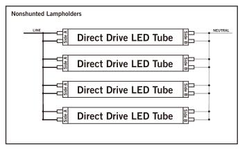
4. Complete all electrical connections with appropriate connectors/wire nuts as needed, per all local and national electrical codes. NOTE: There should not be any exposed wires from sockets left unconnected.
