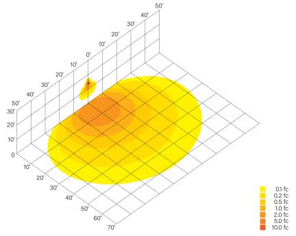
Ground mounted at 6" above ground, 10° above horizontal, shining towards building exterior wall at 14' away
