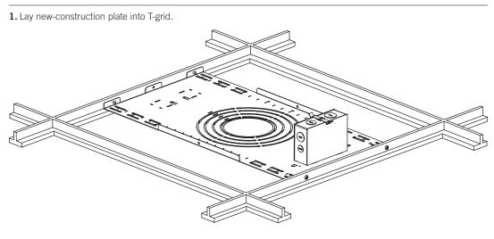
2. Secure plate to T-grid with appropriate screws (not included).
