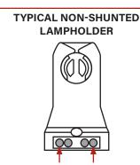
Connect wires directly to these terminals
