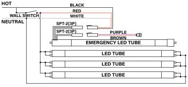
\*Note: Wiring can be configured differently, so long as power is cut to the sockets and the emergency tube wiring is connected to line voltage.
