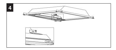
5. Embed the rotary screws on the edge of the panel into the bracket chutes. Push to the end in the direction of chutes to secure panel.
