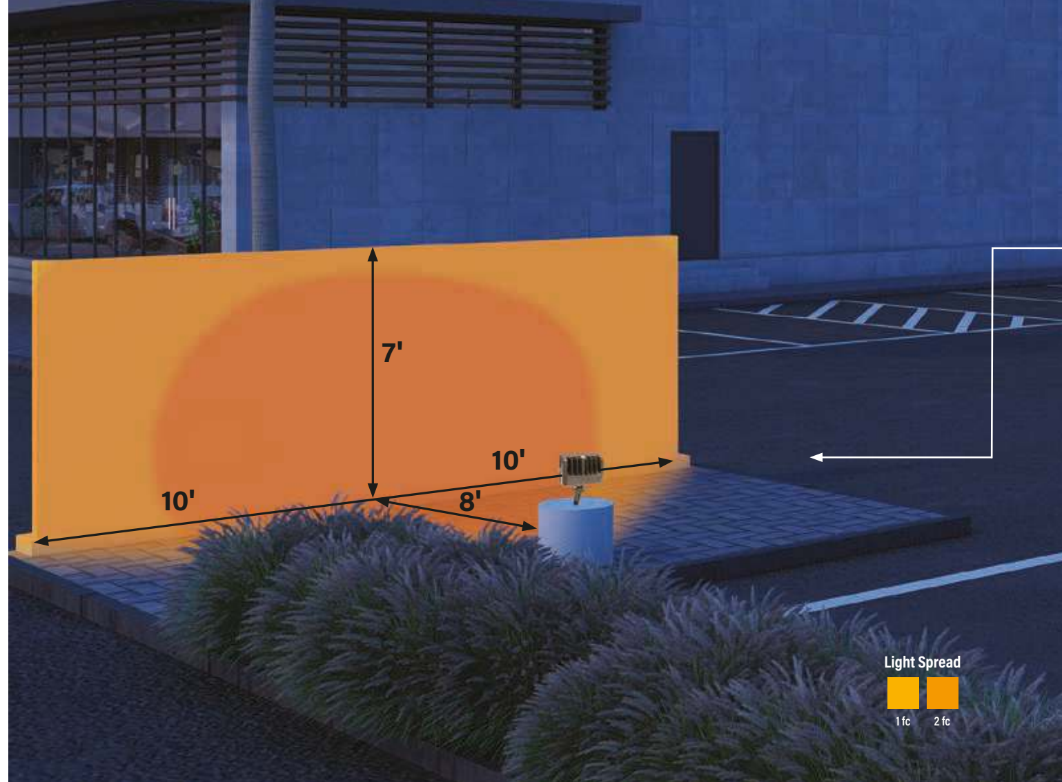
15W Floodlight: Ground Mount at 6" above horizontal; 8' from wall
