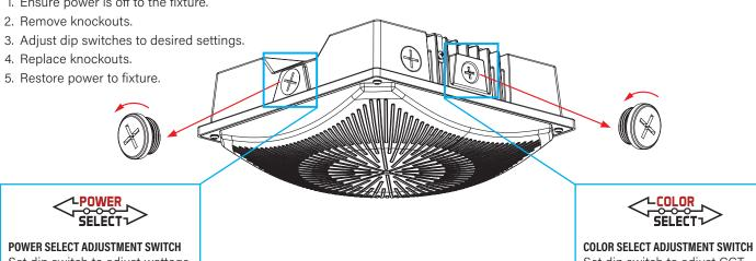
Set dip switch to adjust wattage between 20W, 30W, and 40W. Fixture comes preset at 40W.
